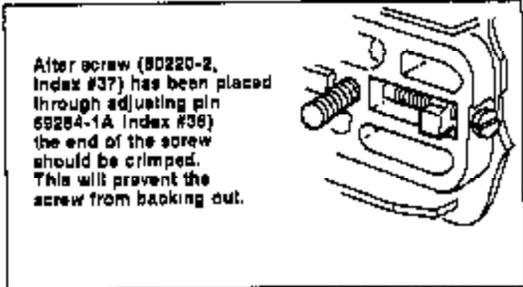
After screw (80220-2, Index #37) has been placed through adjusting pin 69264-1A, Index #38) the end of the screw should be crimped. This will prevent the screw from backing out.
